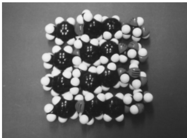
Figure 14. CPK models showing a non-intercalated parallel arrangement of the molecules of compound 4/4 .
